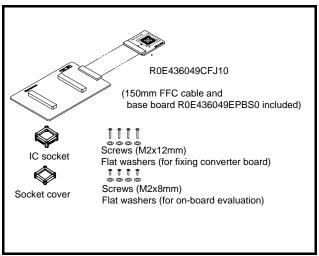
Figure 1 Package components of the R0E436049CFJ10
